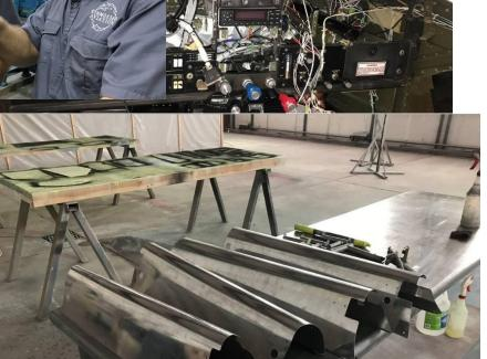
Making a new panel and cutting out all the openings for the glass instruments and backup equipment. Larry is also painting blades for an R66 helicopter and prepping this rotorcraft to be shipped in a container to the Philippines to help another mission who facilitate our organization, as well.
